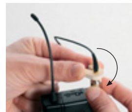
A connector tightening tool is supplied with each adapter and is to be turned clockwise.
