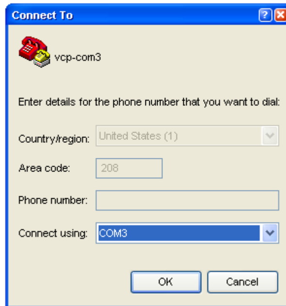
Figure 6-28 Create HyperTerminal for the virtual com port
