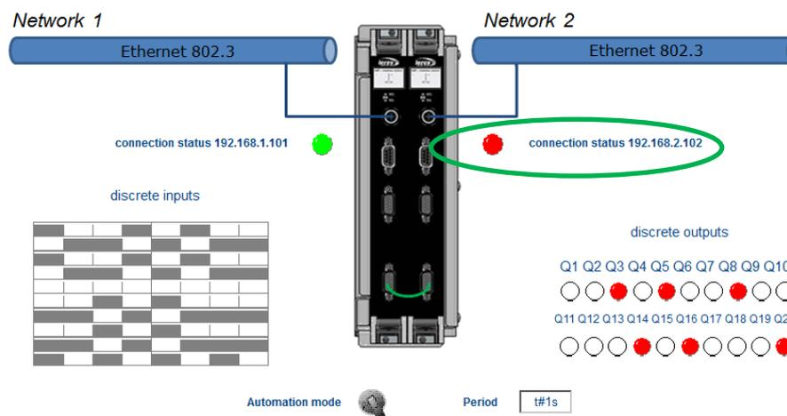
Network 2 disconnected & local link between both BRIO disconnected: management is still OK only on BRIO1.
