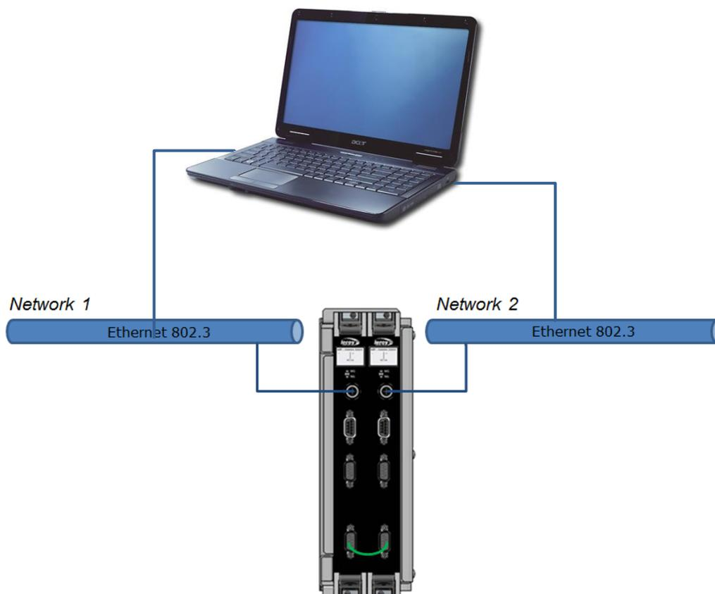
2 projects have been developed with STRATON IDE in order to test both communication types (EtherNet/IP & UDP).
