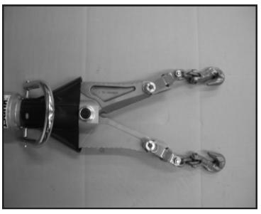
To attach optional chain and shackle accessories for pulling operation, slip tips over the ends of the blades until they are secure.
