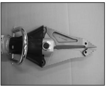
After use, position the blades to a slightly open position for storage. Remove hydraulic pressure from the tool. Move the thumb control in both directions to equalize the pressure. Disconnect the tool from the power unit and connect the two short hoses (pigtails) of the tool to each other. For storage, protect unit from moisture or store in moisture-free location. Secure in adequate storage space to prevent tool damage and kinking of the hoses.
