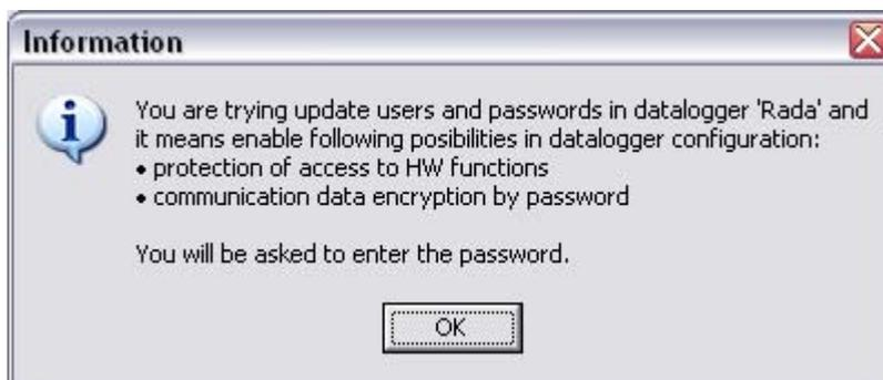
Figure 3: Invitation to enter necessary password for encryption of communication data
