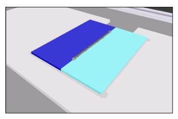
Figure 7-3: Butt Weld
