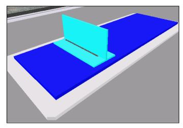
• **T-joint weld:** A T-joint weld is shown in Figure 7-2.
