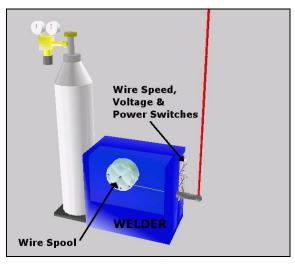
Figure 7-15: Built-in Welder Features
