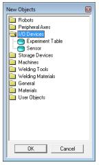
RoboCell I/O (input/output) devices can be connected to any free input/output terminal. The robot controller has eight digital input and eight digital output connections.
