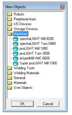
The Machines group includes four Mills (**spectraLIGHT Mill 0200**, **proLIGHT Mill 1000, expertMill VMC-0600, Super proLIGHT Mill 1000**) and two Turns (**spectraLIGHT Turn 0400, proLIGHT Turn 3000**). A CNC controller controls these machines. The robot controller and the machine controller communicate through inputs and outputs. The machine output is the controller input, and vice versa.
