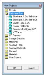
Peripheral devices include a motor with speed and position control. They are connected as axis 7 or axis 8 of the controller.
