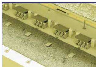
*Fig. 5.5. TE coolers's leads insertion*
