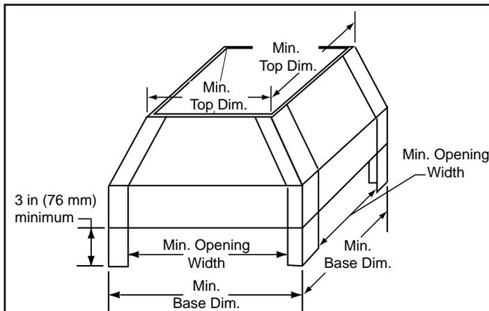
Figure 10.2 Open Top Shroud Dimensions
