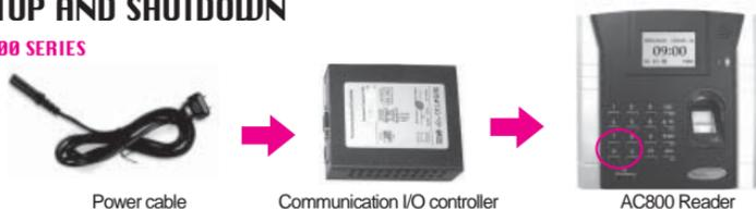
1. Connect the communication I/O controller to the FingerTec® AC800 model.
