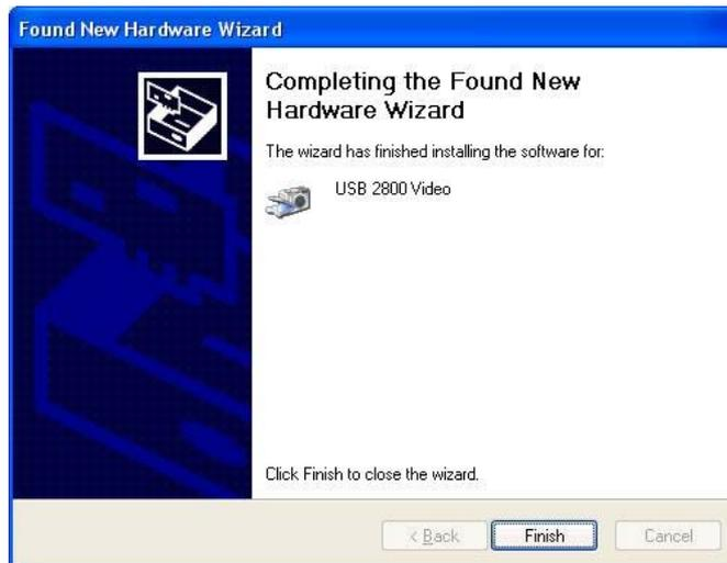
**2.2.11.** Please check GrabBeeX driver was install successful in your computer; (Go to My Computer->Control Panel->System ->Hardware->Device manager->Imaging device")
