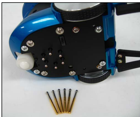
< Spare Part : Power supplying Pin Total 24 ea (4 robots, each 6 pins) >
