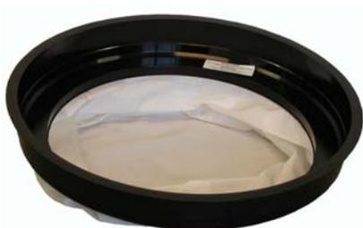
The micro pre-filter is held in place by the filter grid under the motor top. The micro pre-filter holds back the fine and smallest dust particles and protects at the same time the turbine blades of the two suction motors. The turbine blades can be damaged if there are wearing particles in the air current.
