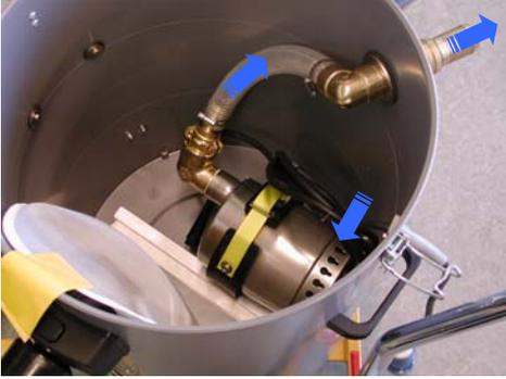
The built-in pump can transport the sucked up and now filtered liquid directly on to drain during operation.
