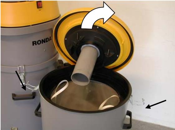
The collection basket in container 1 keeps back the large particles and is emptied when needed. When the collection basket is almost full, the vacuuming is stopped. Let the machine empty container 1 of any liquids before the machine is switched off.
