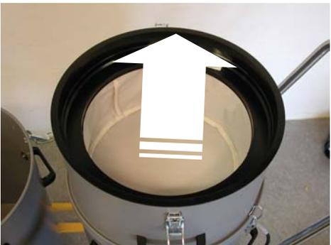
The air is finally filtered by the micro pre-filter, which holds back possible small particles in the air current. In this way you can be sure that the exhaust air has been cleared of dust, which is also an advantage to the suction motors.
