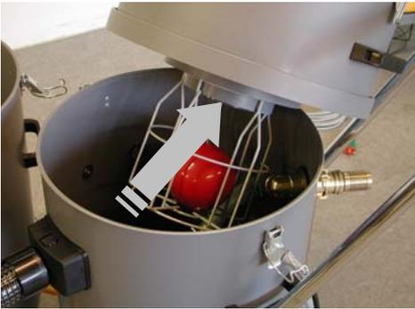
The air current passes the float valve and continues up into the liquid/dust separator.
