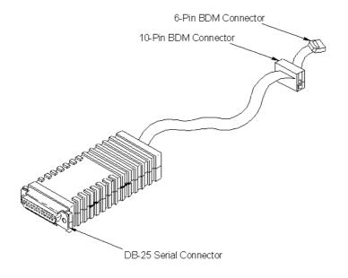
With this interface, you can download an executable program from the HI-WAVE environment to an external target system based on a Motorola MCU which will execute it. You will also have the feedback of the real target system behavior to HI-WAVE.
