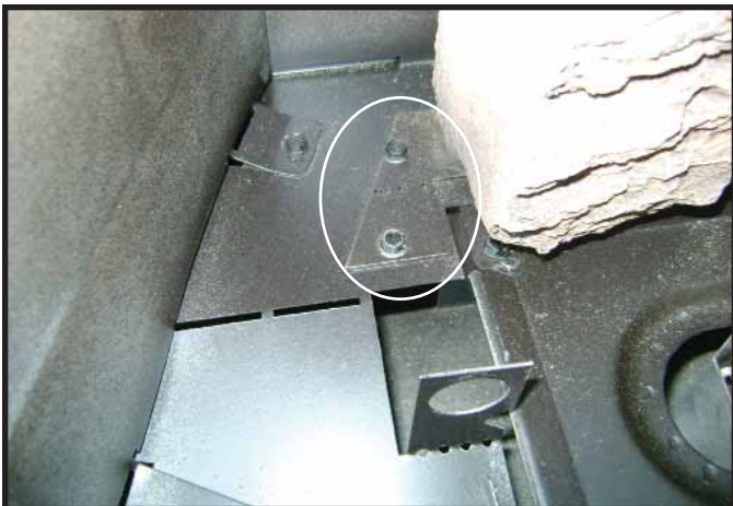
Figure 3.4 Remove Screws from Log Tabs
