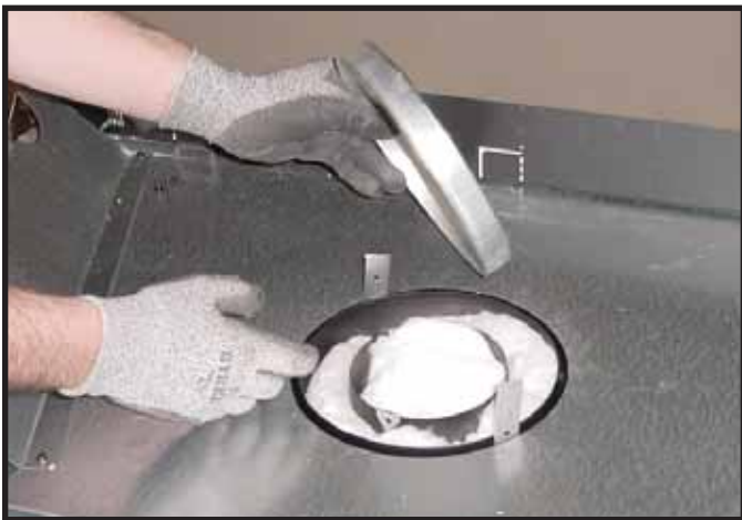
Figure 9.3 Remove the seal cap.
