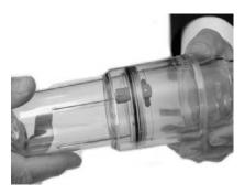
**STEP 12.** Verify the oversized O-ring slips in place and looks as shown.
