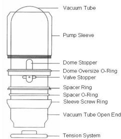
**STEP 4.** Move the PUMP SLEEVE up and down while turning it back and forth. This causes the oil to seep onto the O-RING.
