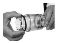
**STEP 14.** Slide the black sleeve (thicker) O-ring (oiled) onto the main cylinder behind the spacer ring.
