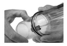
**STEP 6.** Place oversized (thinner) O-ring in groove between valve & dome stopper as shown.
