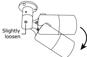
Step2: Adjust the viewing angle of the camera, as indicated below.
