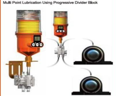
Remote multi point lubrication is available with the micfil automatic lubricator using a divider block. It is recommended to test the back pressure of the bearing, lube lines, and divider block after assembly using a grease gun connected to a pressure gauge. Ensure the break-off pressure is below the average operating pressure of 30kg/cm² (425psi).
