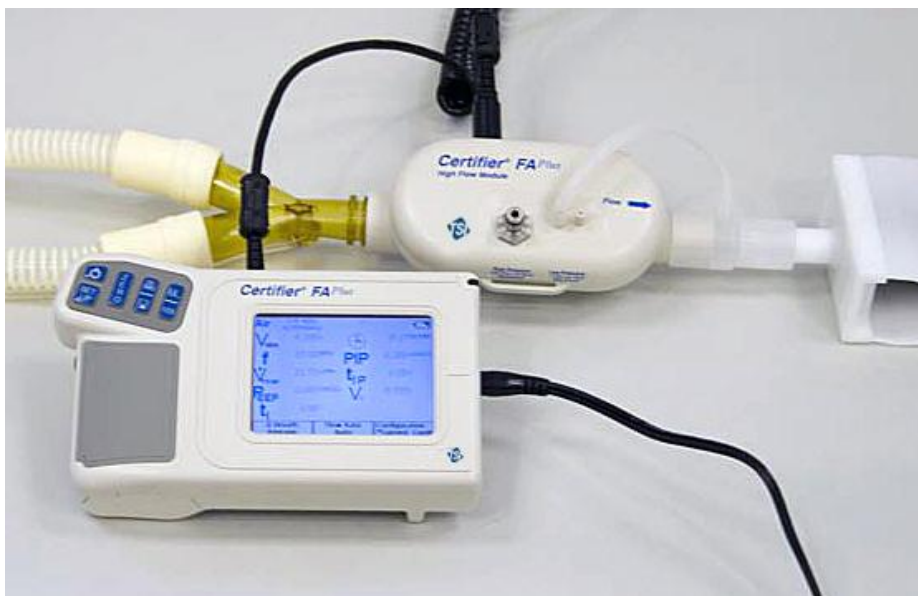
Figure 11. Installing a Flow Module into the Circuit for Measuring Bi-directional Flow (flow direction Arrow should be towards test lung)
