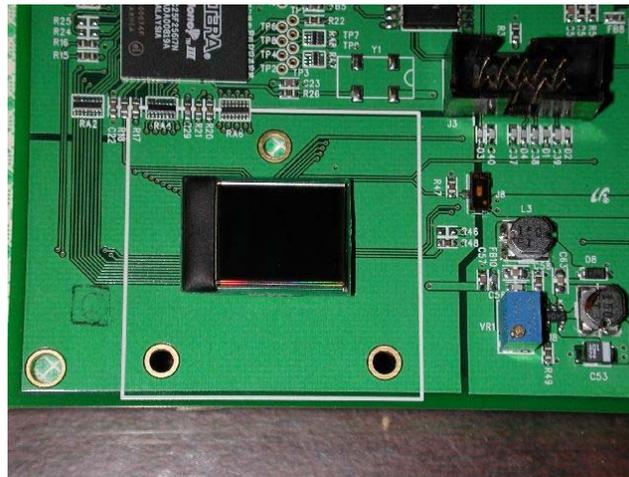
*Figure 4-1 Display Carrier Board Connection Orientation*
