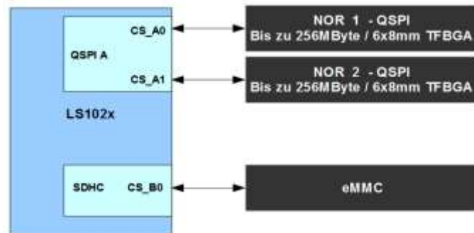
Illustration 8: On-board flash maximum expansion
