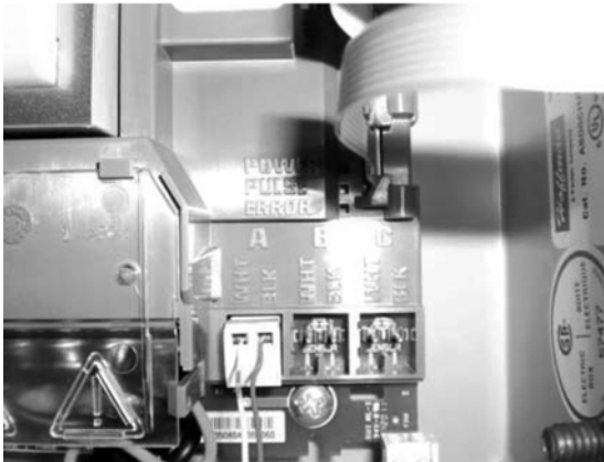
Fig. 10. Sensor Polarity. When current sensor is installed properly, error LED is off. If the Error LED is illuminated, then disconnect the gray plug and reverse the input lead. If it clears, the "Sensor Error" then mark appropriately. Repeat for all sensors.
