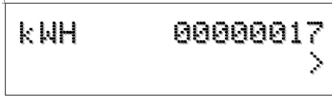
Fig. 15. The Class 1000 kWh meter displays readings in whole numbers, there are no decimals.
