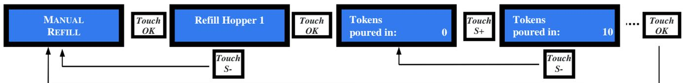
When touching the S+ button, quantity goes 10 units up; touch repeatedly until reaching the desired figure (max. available is 2500 units). If the S+ button is maintained pressed, the count-up will be as fast as 100 units/second (2500 units in 25 seconds).
