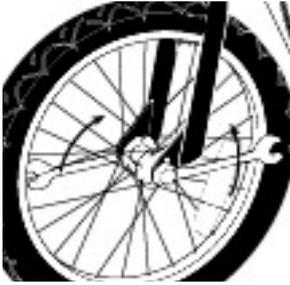
**1** Loosen front axle by attaching 10/15 mm wrenches to both axle nuts and loosening counter-clockwise.
