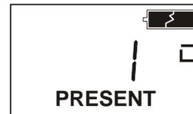
Fig. 12. T7270A and RT7070A taught-in for room #1; battery level OK
