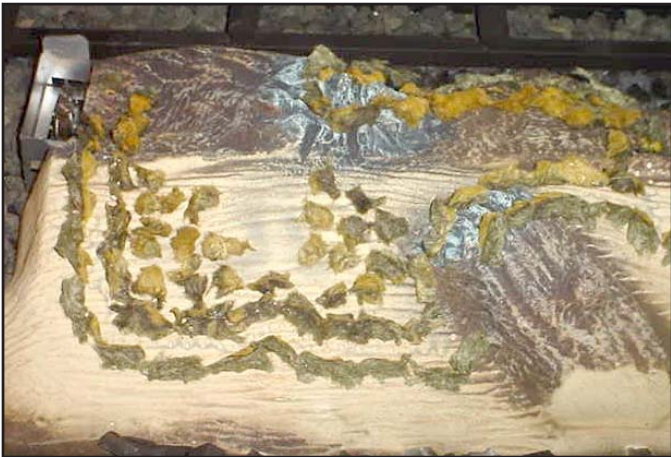
Figure 50. Placement of the Ember Material
