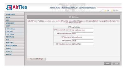
After you click "Save", you will be asked to confirm that you would like the information to be saved in the device. After clicking OK, the VoIP LED on the front panel of the WAV-180 will turn on. In addition, "SIP Server Registration State" will become "Registered" in the "VoIP Service State" window.
