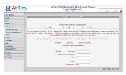
802.1x is a port-based access control in which the wireless clients are authenticated by a central RADIUS server. If you have a RADIUS server in your network, WAV 180 can defer the authentication function to this server at the IP address you provide. Otherwise, it should be left alone.
