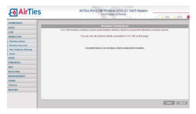
To configure your wireless network, go to "Wireless Settings" under the "WIRELESS" menu on the left menu bar of the AirTies WAV-180 Web interface. In the "Wireless Settings" screen, verify that the wireless network feature is activated. Wireless network is active by default.
