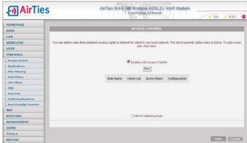
After checking the "Enable LAN Access Control" box, click "New" to define a new access rule.
