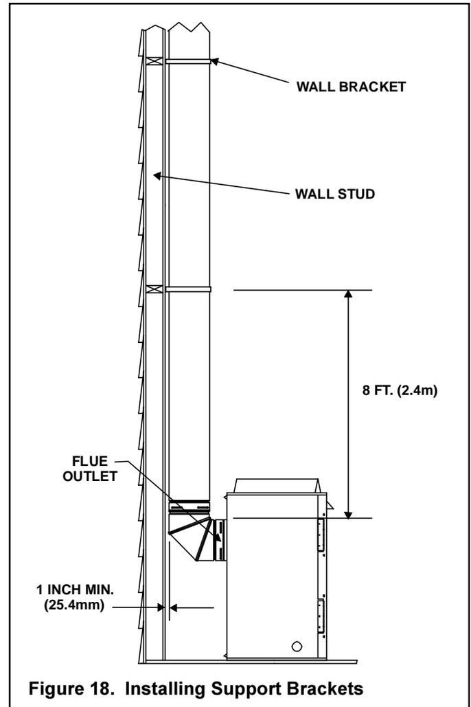
Figure 18. Installing Support Brackets
