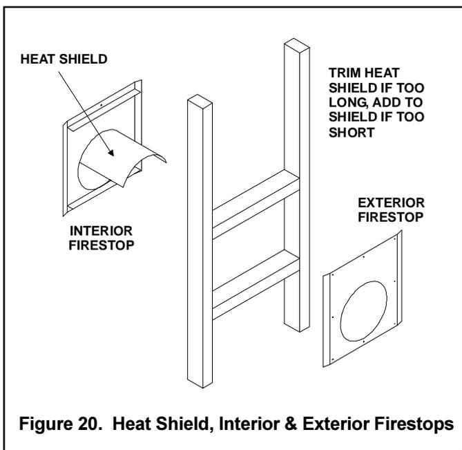
**Figure 20. Heat Shield, Interior & Exterior Firestops**
