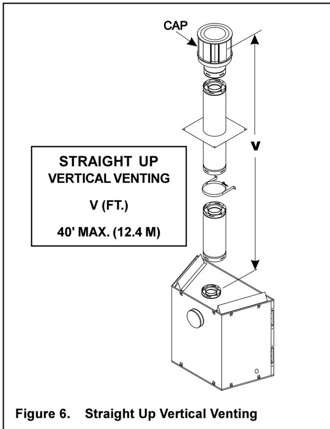
**Figure 6. Straight Up Vertical Venting**
