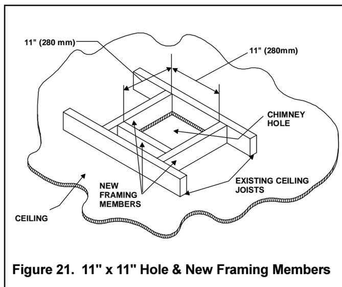
**Figure 21. 11" x 11" Hole & New Framing Members**
