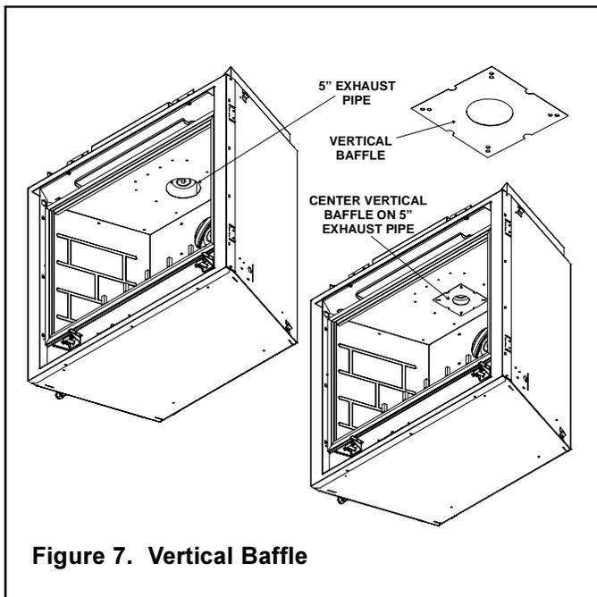
**Figure 7. Vertical Baffle**
