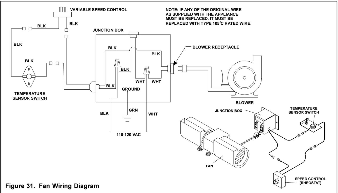
Figure 31. Fan Wiring Diagram
