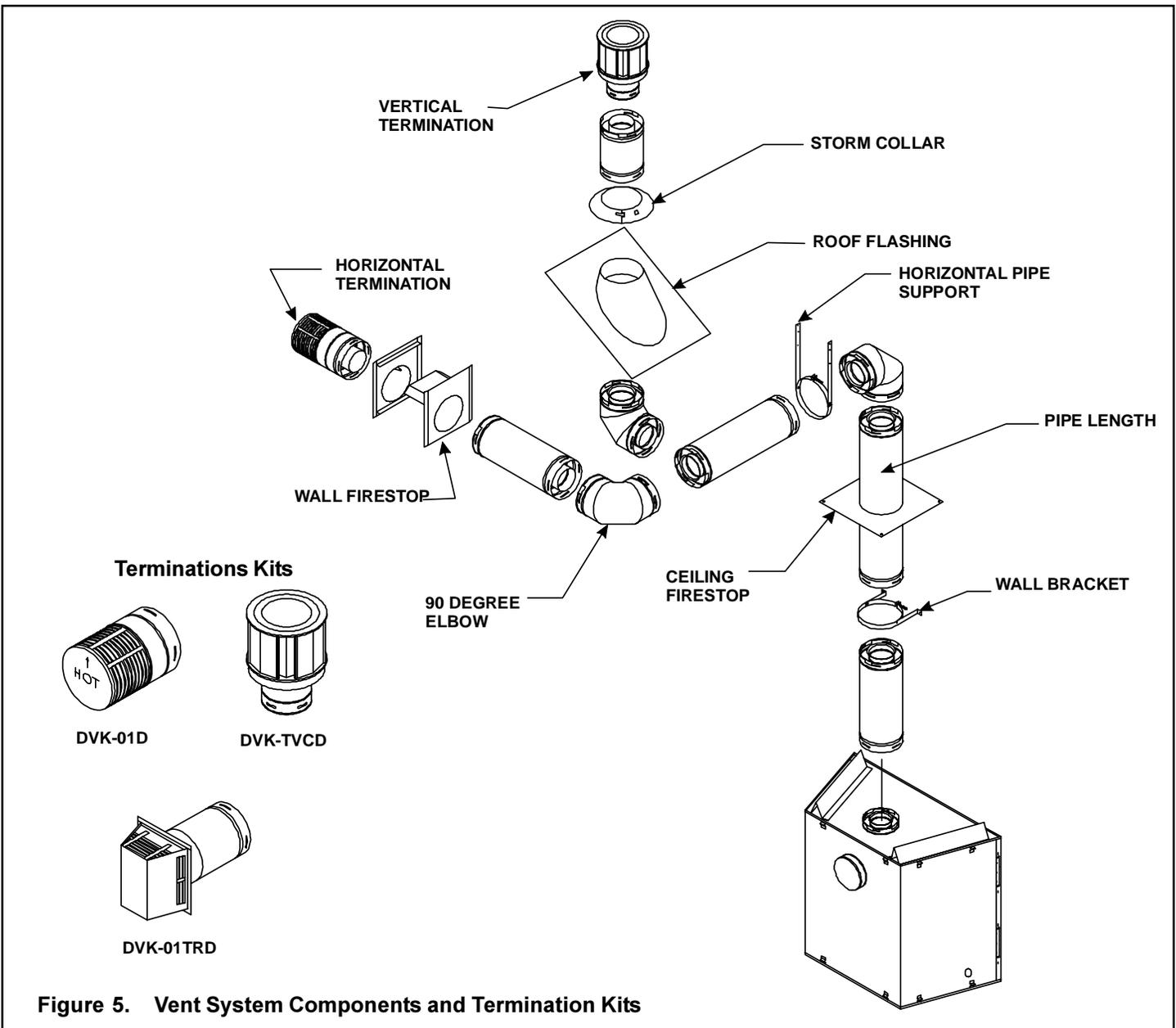
Figure 5. Vent System Components and Termination Kits
