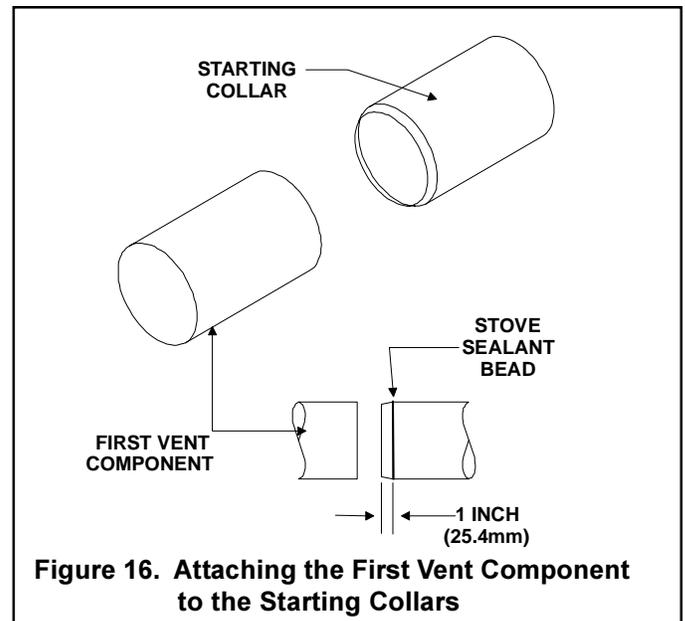
Figure 16. Attaching the First Vent Component to the Starting Collars
