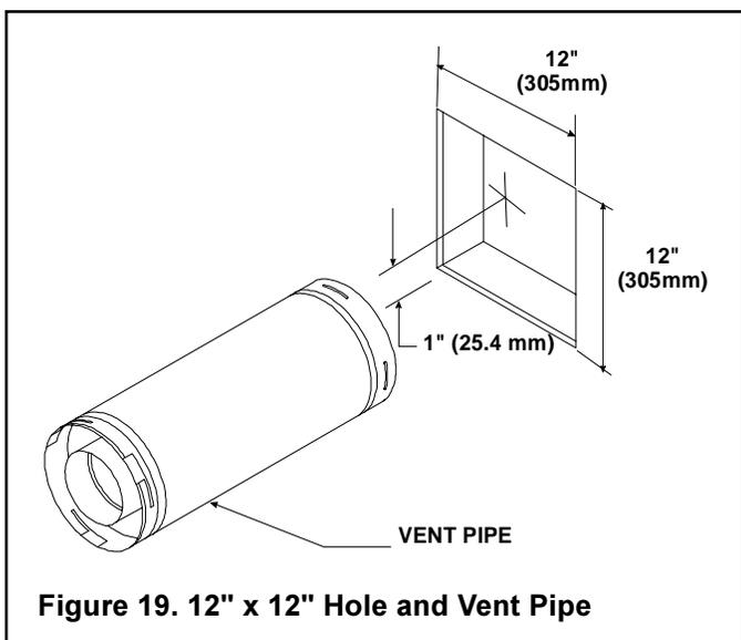
**Figure 19. 12" x 12" Hole and Vent Pipe**
