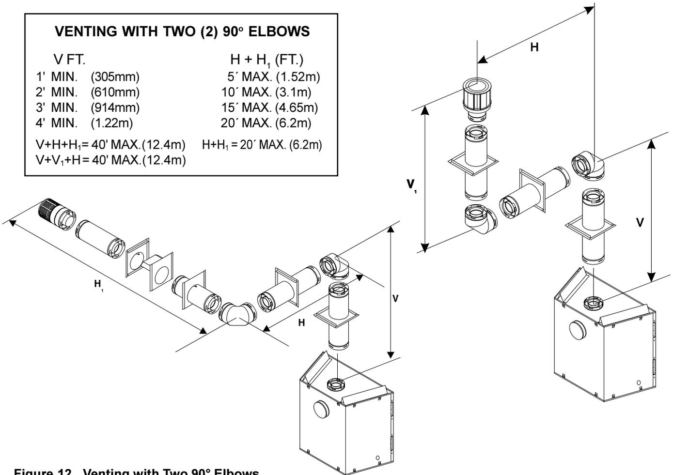
**Figure 12. Venting with Two 90° Elbows**
