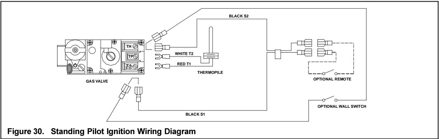
Figure 30. Standing Pilot Ignition Wiring Diagram
