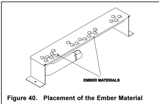
Figure 40. Placement of the Ember Material
