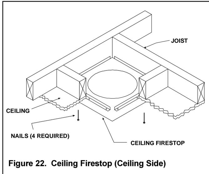
**Figure 22. Ceiling Firestop (Ceiling Side)**
