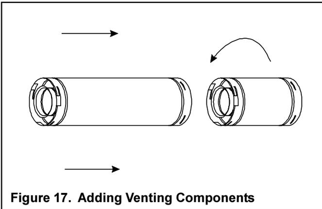
Figure 17. Adding Venting Components
