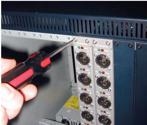
Securing a Stage Rack option card to the Stage Rack front panel (SRO card shown)
