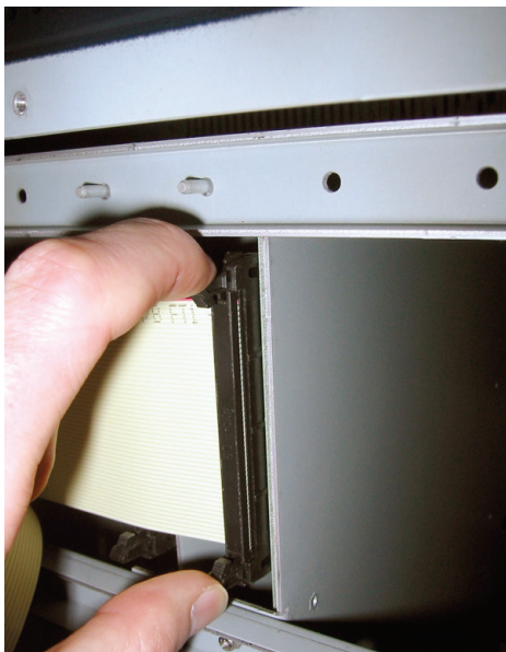
Connecting a Stage Rack option card to the Stage Rack ribbon cable
