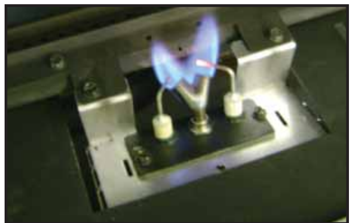
Figure 3.1 IPI Pilot Flame Pattern
