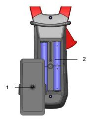
Figure 6: The Battery Compartment
