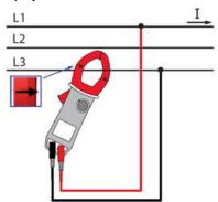
**NOTE:** 3-phase power on a balanced 4-wire network can also be measured by proceeding in the same way, or by proceeding as for the measurement on a single-phase network, then multiplying the value by three.
