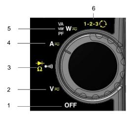
Figure 2: The Function Rotary Switch
