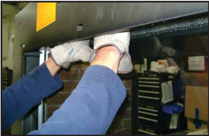
Figure 14.6 Top Glass Latch Access
