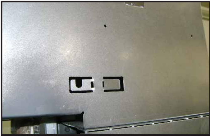
Figure 14.28 Mesh Rod Support Tabs
