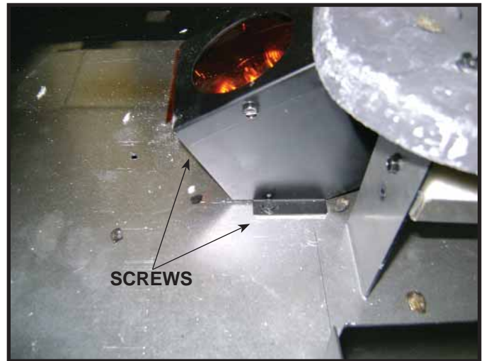
Figure 14.11 Light Housing Removal
