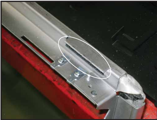
Figure 14.1 Glass Top Tab Detail.
