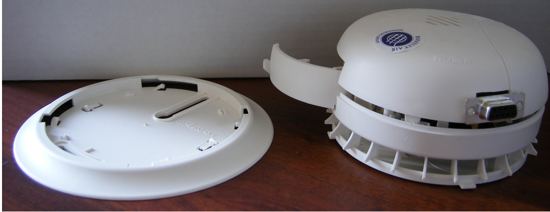
Figure 2. Space created by loosening the UCB PM lid from the base. Note – the baseplate, used for mounting the monitor on a wall, must be removed before you can access the tabs to remove the UCB PM lid.
