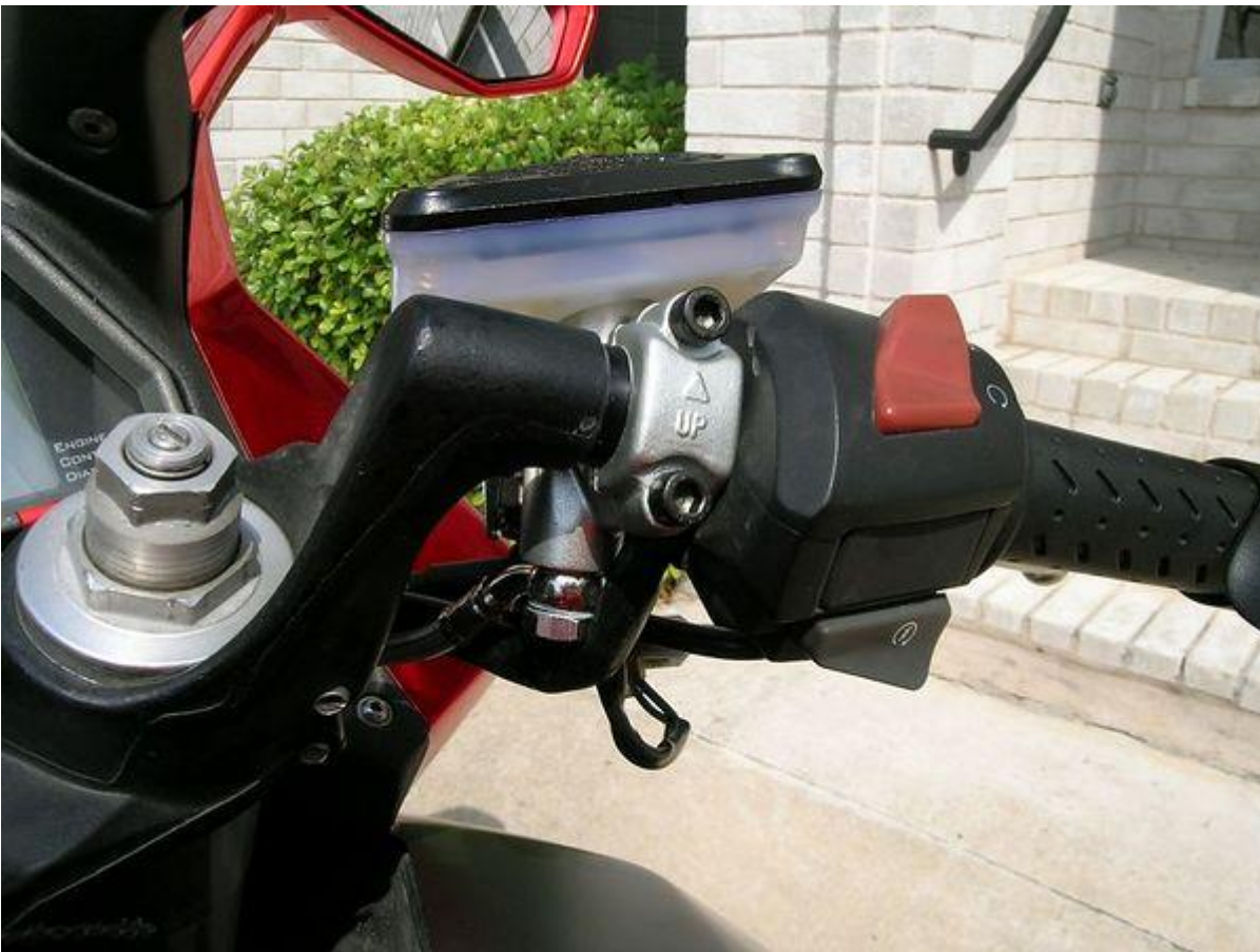
Brake switch ( much nicer than the problematic stocker). These wire connections are pre-production; see next photo for the production version.
