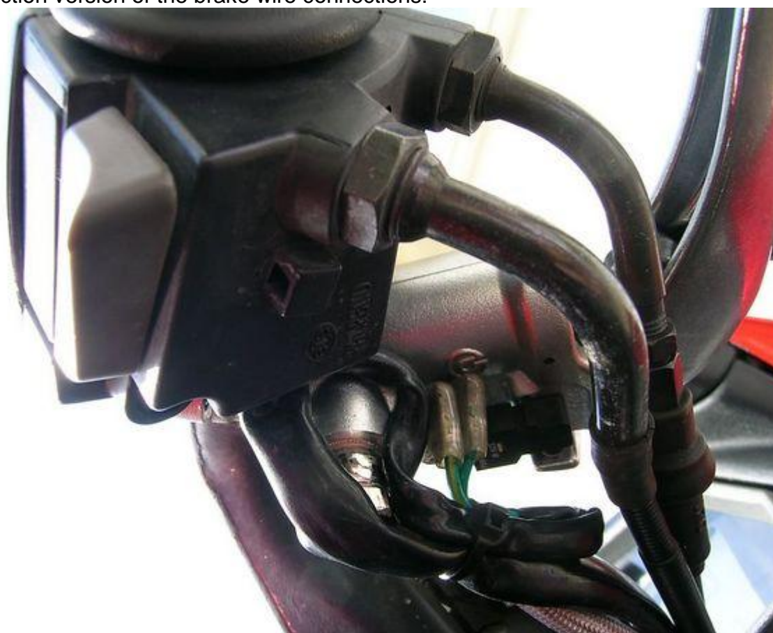
The levers have a bit of adjustment, as you can see: I measured 15mm for the brake, and 5mm
