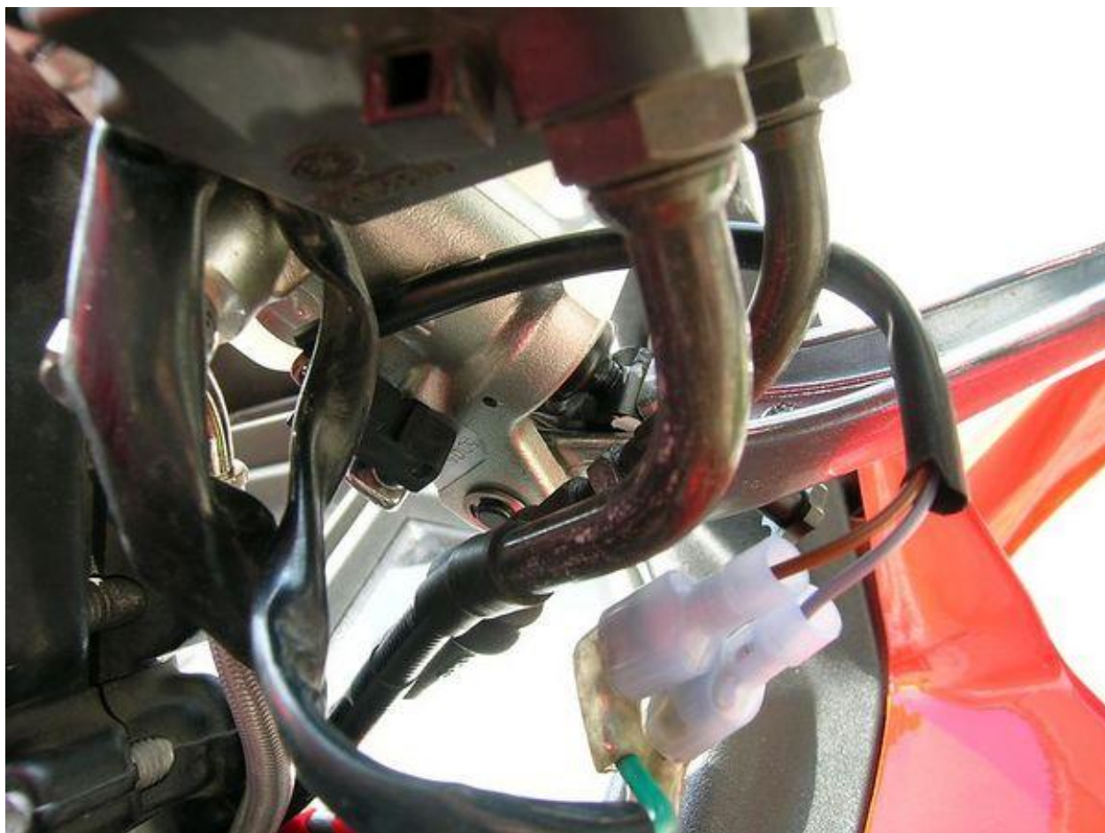
Production version of the brake wire connections:
