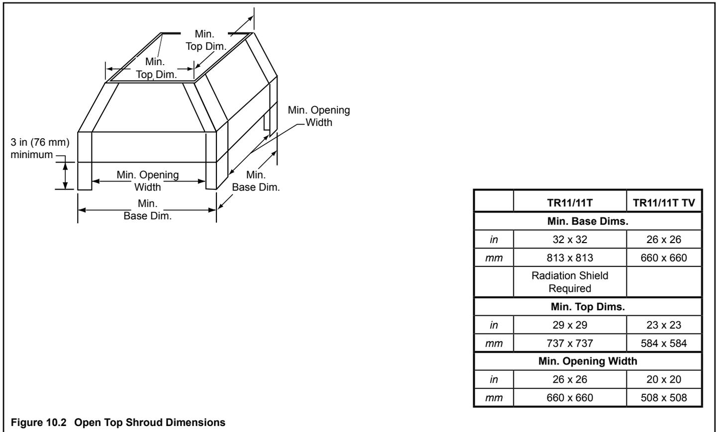
Figure 10.2 Open Top Shroud Dimensions
