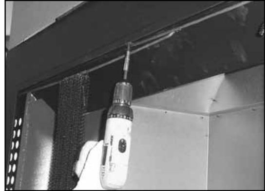
Figure 7.3 Remove Screen Rods
