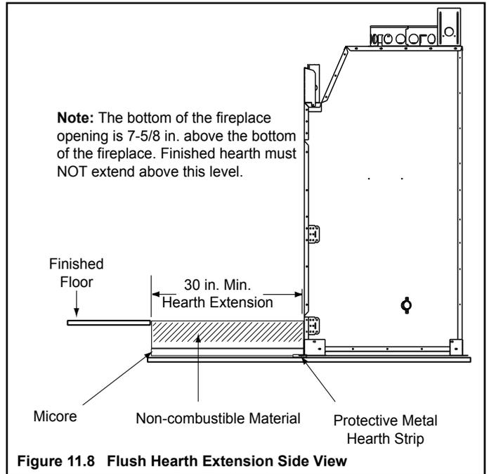
Figure 11.8 Flush Hearth Extension Side View
