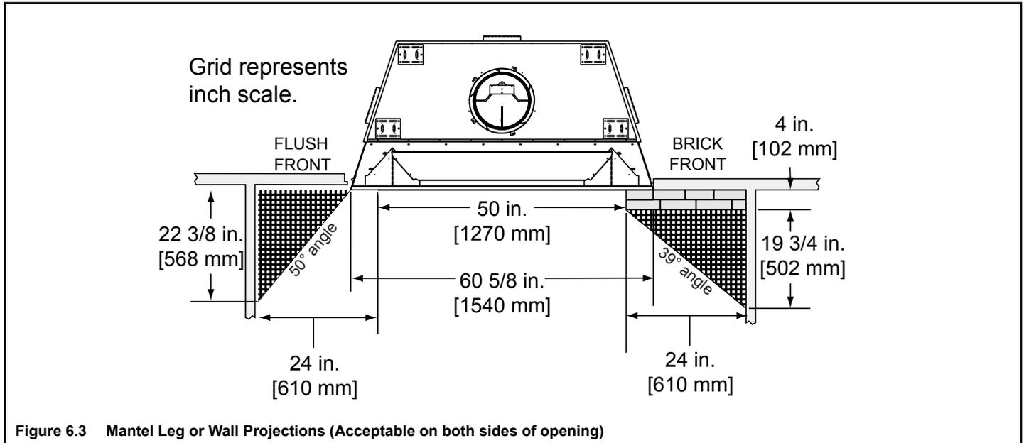
Figure 6.3 Mantel Leg or Wall Projections (Acceptable on both sides of opening)
