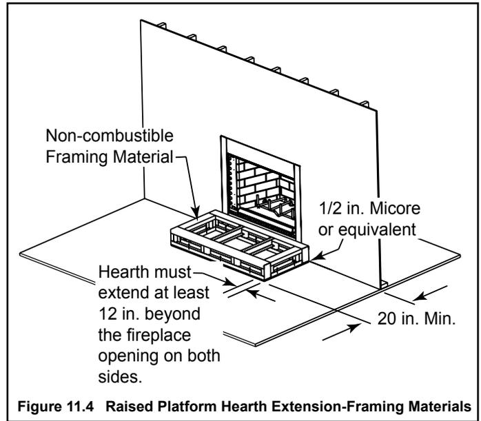
Figure 11.4 Raised Platform Hearth Extension-Framing Materials
