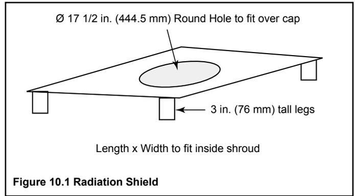
Figure 10.1 Radiation Shield
