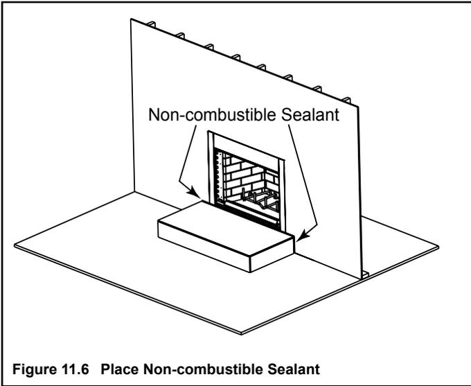
Figure 11.6 Place Non-combustible Sealant
