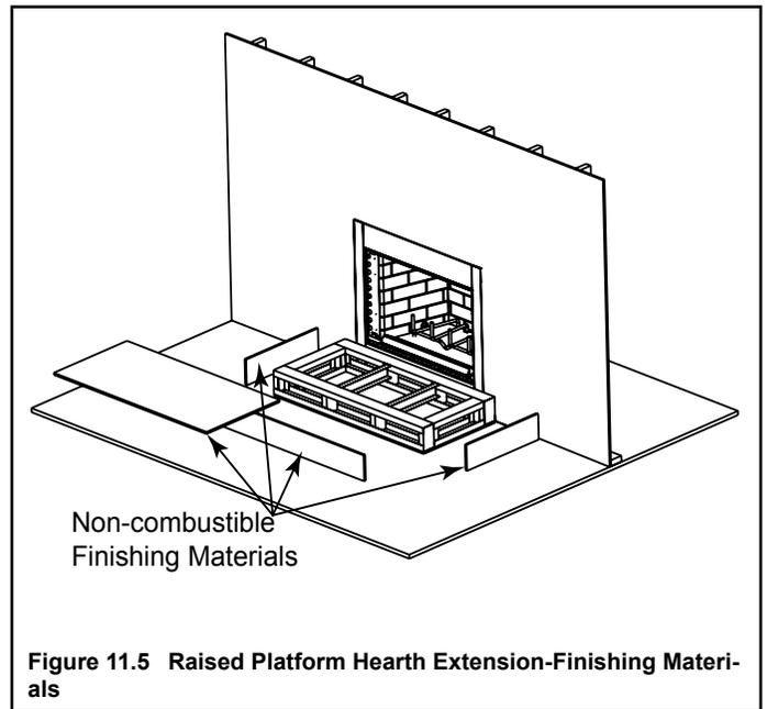
Figure 11.5 Raised Platform Hearth Extension-Finishing Materials
