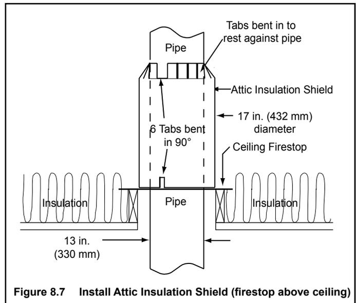
Figure 8.7 Install Attic Insulation Shield (firestop above ceiling)
