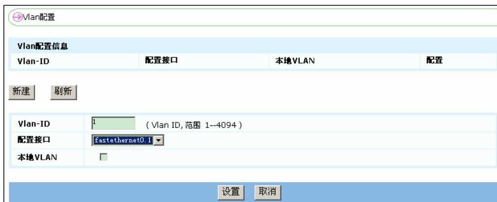
Input 1 in the Vlan-ID box, select fastethernet0.1 as the configured interface, and click Set to add a VLAN.
