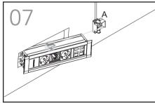
Using a very fine-tipped screwdriver, remove the covers that protect the anchor system.
