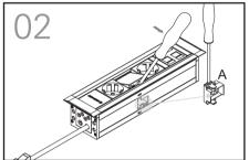
**IMPORTANT**: Using a very fine-tipped screwdriver, remove the covers that protect the anchor system.
