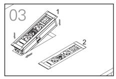
Insert the power cable first and then insert the profile frame as shown in fig. 3.
