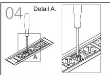
Using a Phillips head screwdriver, tighten the two anchor screws until they are tight enough to prevent movement.
