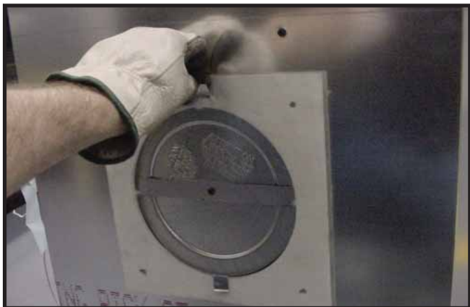
Figure 9.8 Fold the tabs toward the center of the seal cap (90°) and remove the insulation gasket.
