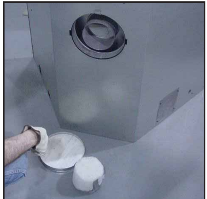
Figure 9.11 Discard the vent cap, remove and discard the insulation basket.
