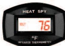
TEST mode flashes room temperature to show Heat Spy is working properly.
