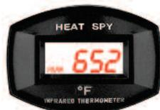
PEAK holds highest measured temperature, and is especially useful in high temperature scans.
