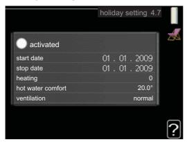
To reduce energy consumption during a holiday you can schedule a reduction in heating, ventilation and hot water temperature.
