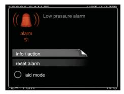
In the event of an alarm, some kind of malfunction has occurred, which is indicated by the status lamp changing from green continuously to red continuously. In addition, an alarm bell appears in the information window.
