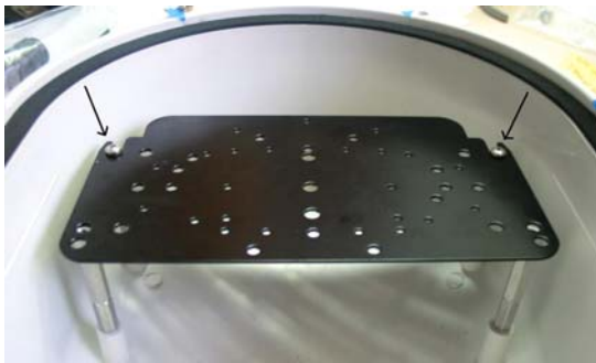
Picture represents standoff location & camera bracket orientation. Height of standoffs will vary depending on camera used.
