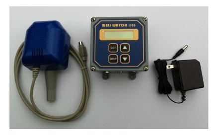
The Well Watch 1100 is a simple to use self-contained portable acoustic ranging instrument designed specifically to find the distance through a well casing or sounding tube to the water surface. However, it also can be used to measure any closed pipe, straight or crooked.
