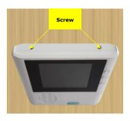
(10) Put the rubber stopper in to the screw hole.
