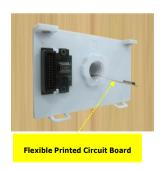
(7) Buckle the connector to connect the adapter plate and outdoor host. (The FPC contains explicit circuit, please don't use too much power to buckle it, or it may destroy the circuit board of FPC or the connector.)
