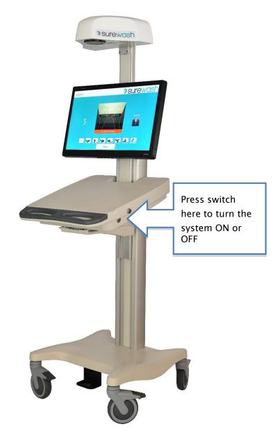
To turn off the system, press and hold the on/off button until the system shuts down. When the system has completely shut down (this takes approximately 30 seconds) the unit may be unplugged from the mains power. SureWash should not be unplugged from the mains power before being shut down.
