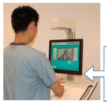
Location of screen ON/OFF button. It is not necessary to turn off the screen seperately and it should not be used in normal operation
