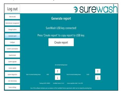
following screen will appear. The 'Create report' button cannot be pressed unless the licence for the system is valid (see section 4.11) and until the SureWash USB key is connected to the system. After plugging in the SureWash USB key, the 'Create report' button can be pressed.
