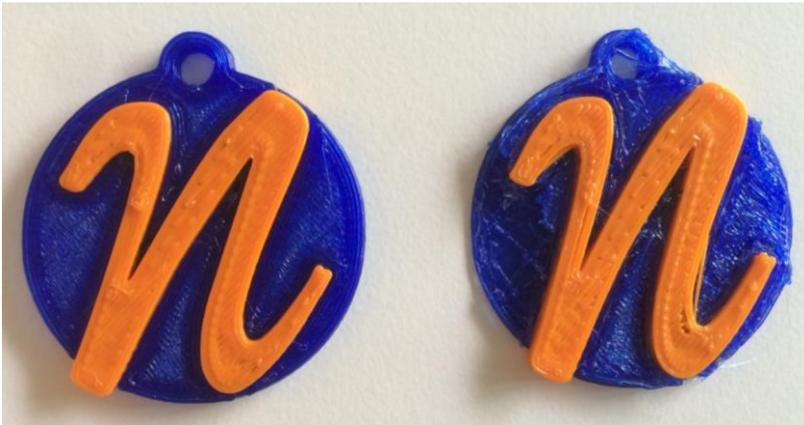
Sample with/without maximal Skirt height on the outside of the model
