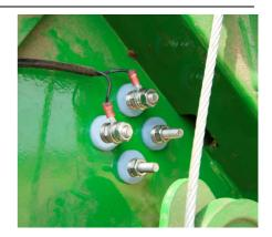
Keep in mind that the cable must be so long that the plug in the attached state is in the cab of the tractor. The excess cable length best to be fixed at a sheltered position at the press. The cable should not be reduced.
