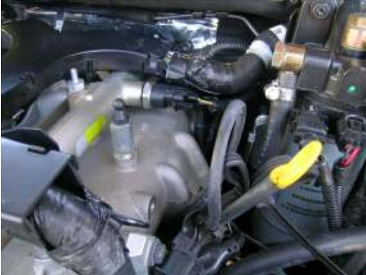
MAP sensor is located on top of the of the intake manifold towards the rear of the engine on the driver's side. The intake manifold is located on top of the engine. It may be necessary to move the plastic race that holds the harness on top of the engine up in order to reach the Map sensor connector. Plug the supplied MAP sensor
