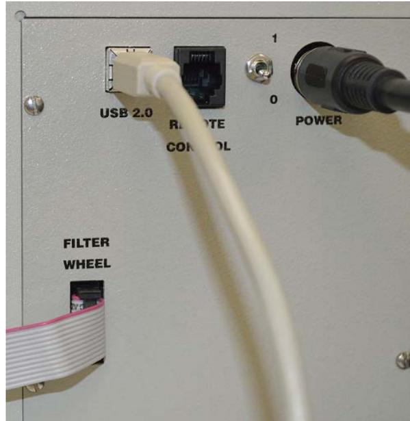
**Figure 6: Monochromator Connections**
