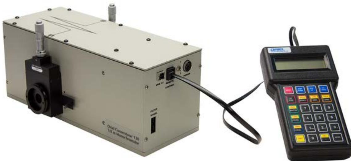
**Figure 24: Cornerstone 130 Monochromator with 74009 Hand Controller**
