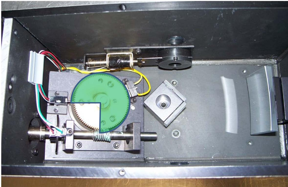
**Figure 30: Grating Turret Position Sensor Pin Range**
