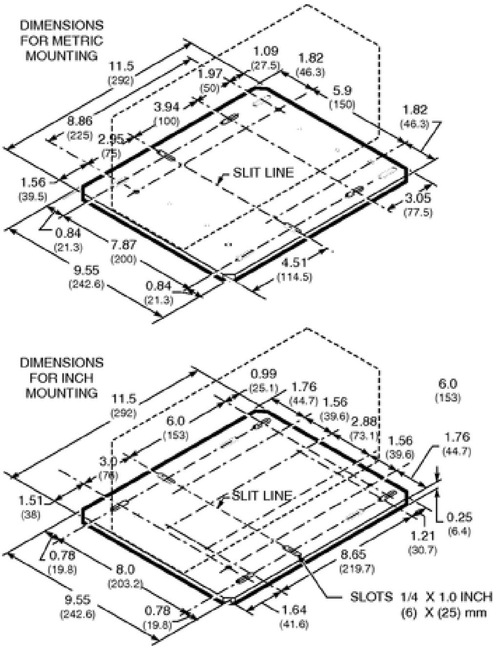
Figure 33: Model 74006 Mounting Plate
