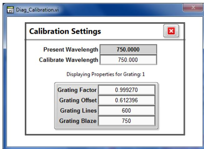
Figure 29: Entering Calibration Values in Utility Software
