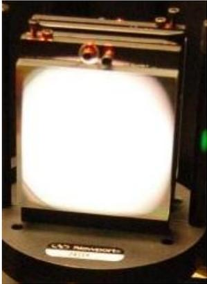
Figure 19: Grating Correctly “Filled” with Light
