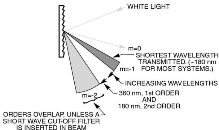
Figure 38: Polychromatic Light Diffracted From a Grating
