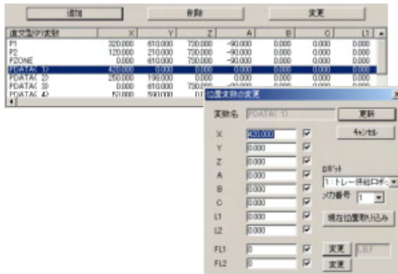
Fig. 5-36 Changing the position array variable (E1 版)
