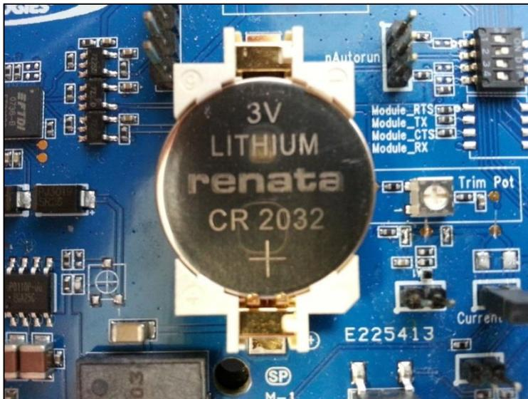
Figure 15: Inserting the coin cell (step 2)
