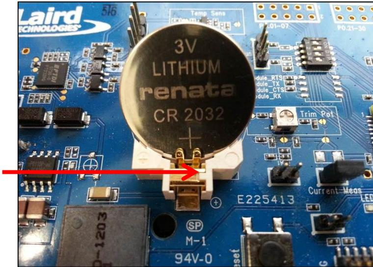
Figure 14: Inserting the coin cell (step 1)
