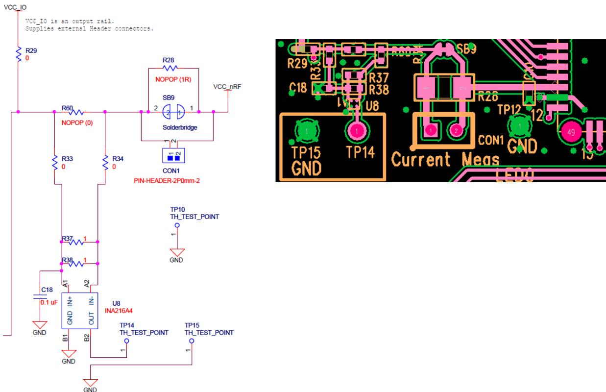
Figure 13: Current measurement Schematic and component location
