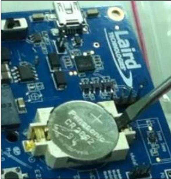
*Figure 16: Removing the coin cell (step 2)*
