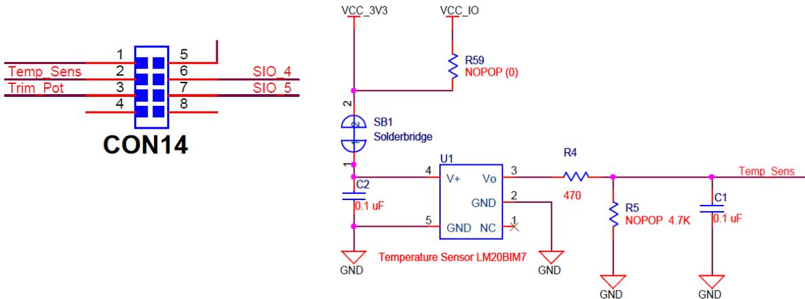
Figure 10: Temperature Sensor
