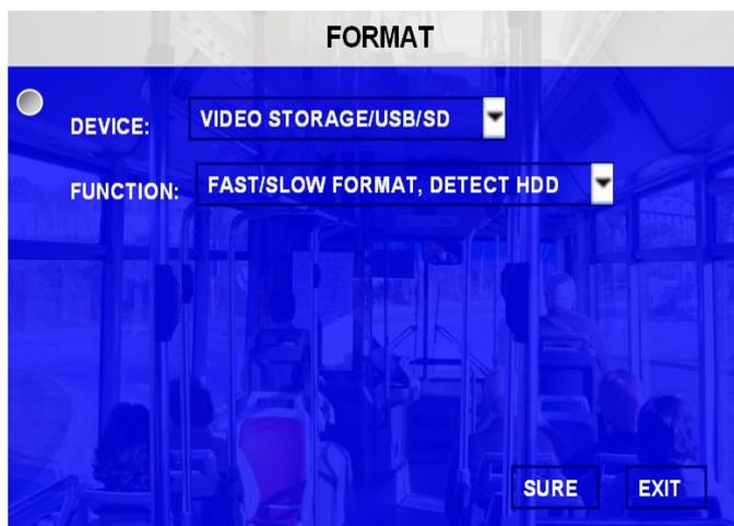
**DEVICE:** Please press **【ENTER】** to select the target device for format. There are 3 options: VIDEO STORAGE, SD and USB. Then press **【FORMAT】** to format the device.
