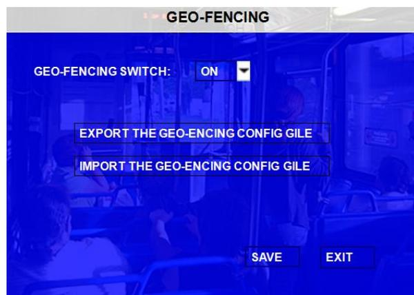
**GEO-FENCING SWITCH:** this is the enable switch for GEO-Fencing function. This switch is only for MDVR terminal.
