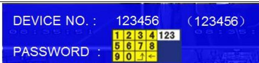
**DEVICE NO.:** The unit ID of MDVR. You can setup the ID for the MDVR in the menu yourself. After setting, the ID number will appear automatically on the login screen. It's the number in the bracket
