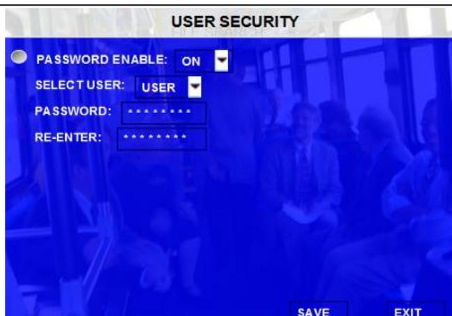
**PASSWORD ENABLE:** To active this function or not. Selecting “ON” will require a password in order to access the setup menu. Selecting “OFF” will not require a password in order to access the setup menu.
